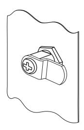
2 Insert the new lock housing into the door hole. Then, insert the lock bracket onto the lock housing from the back of the door and secure using the large nut.
